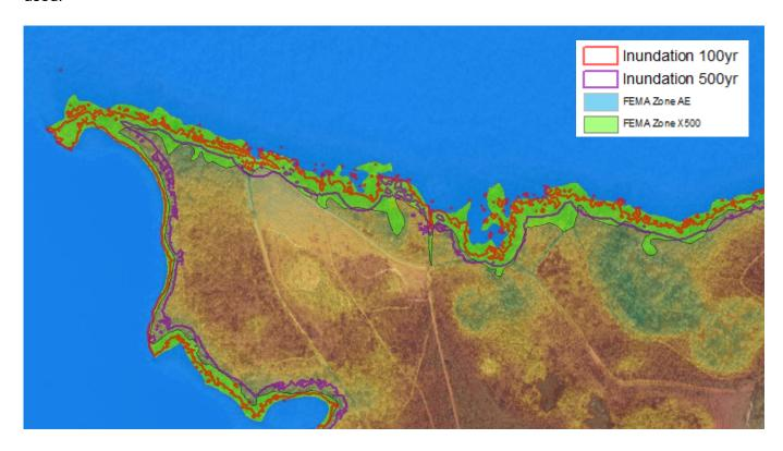
Figure 45. St. Johns River 100 and 500-year Inundation Comparison
