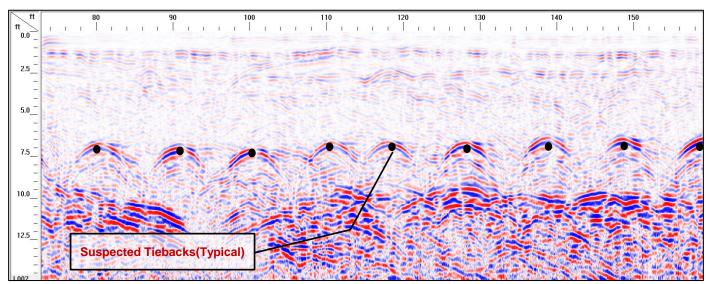
**Transect T-6** - Example GPR profile approximately 25 feet west of the seawall (north to south direction). Tiebacks spaced approximately 10 feet on-center. The depth shown is approximate.
